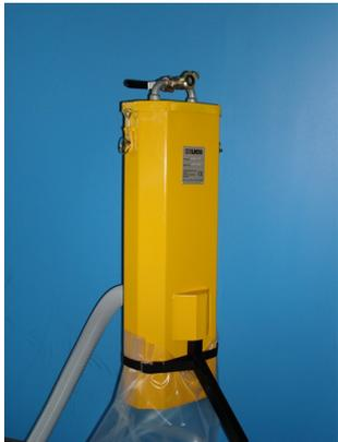
The compact design makes the MACRO light weight and easy to move and carry. During use the MACRO is positioned on a sturdy stand which allows easy access for changing the plastic bag which collects the rock cuttings and dust.
